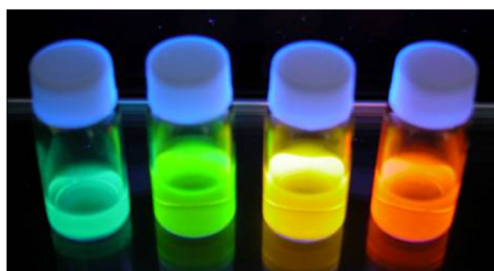
Fig. 3 Fluorescence emission photographs in long UV light of 6a-6d dye in DCM solvent
